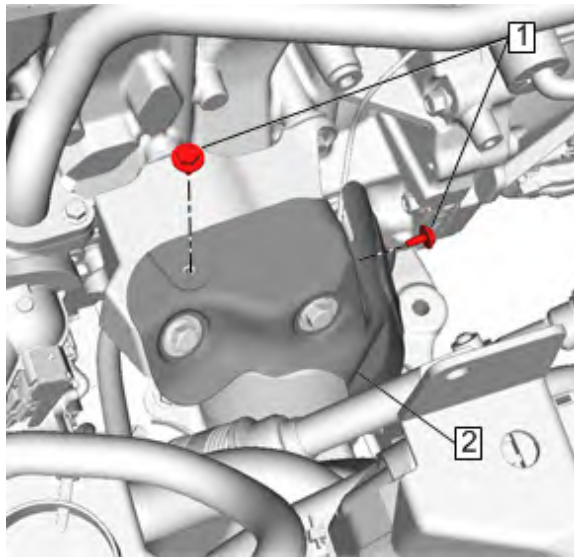
Fig. 47: Engine Mount Heat Shield Fasteners Courtesy of GENERAL MOTORS COMPANY
